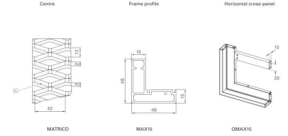
Min./Max. dimensions Width: 550 to 1500 mm
