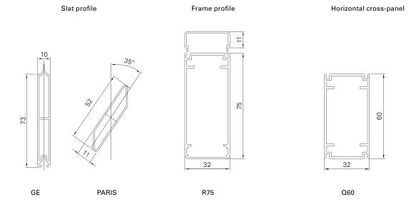
Min./Max. dimensions Width: 280 to 800 mm
