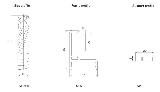
Min./Max. dimensions Width: 550 to 1600 mm
